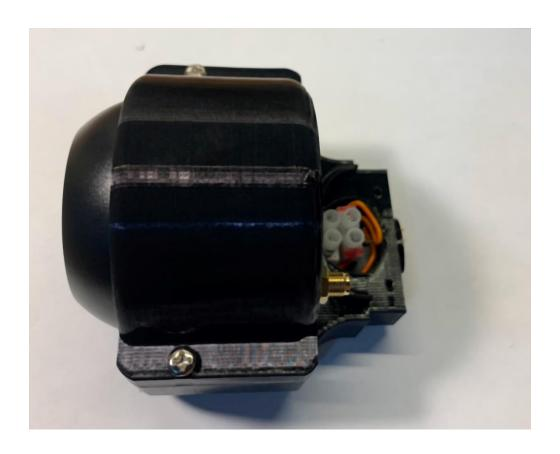
Next remove the orange marker lens from the Furrion maker light on the RV. There are slots on the top and bottom where you can gently pry with a flat screwdriver to remove.
