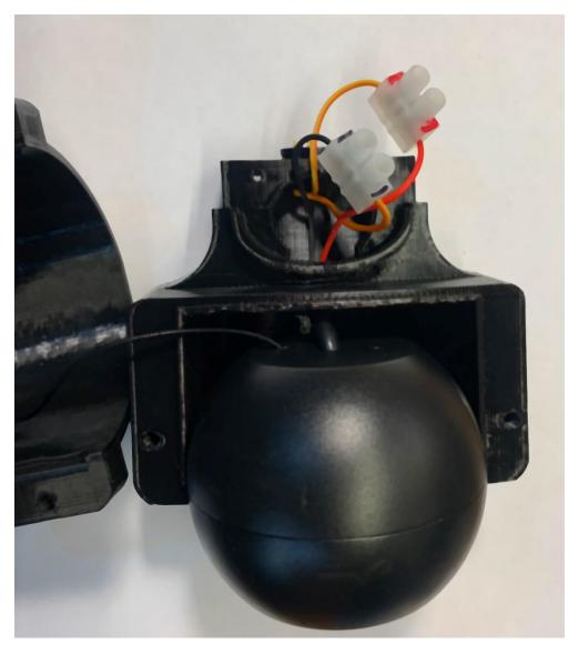
Use care to install the terminal blocks in the hole. No wires should be routed under the terminal blocks to ensure they will have clearance. Set the camera in the saddle mount on top of the rubber pad.
