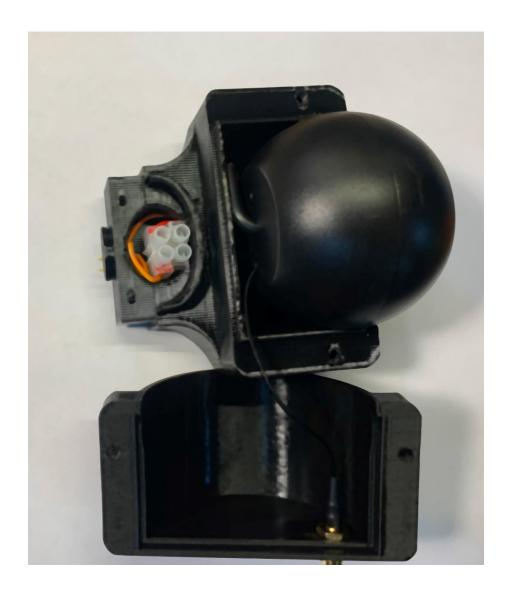
Install the top of the camera adapter. Ensure the power wire and the antenna wire are routed just behind the camera before securing. Hold the top and insert the 2 screws from the original camera housing and snug. Do not over tighten the screws.
