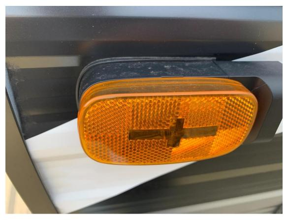
Remove the 2 square head screws that hold the adapter blank to the marker lens and remove the blank by pulling it to the rear of the RV. Remove the Oring from the adapter blank and install it on the DSP Camera Adapter on pin extension area.
