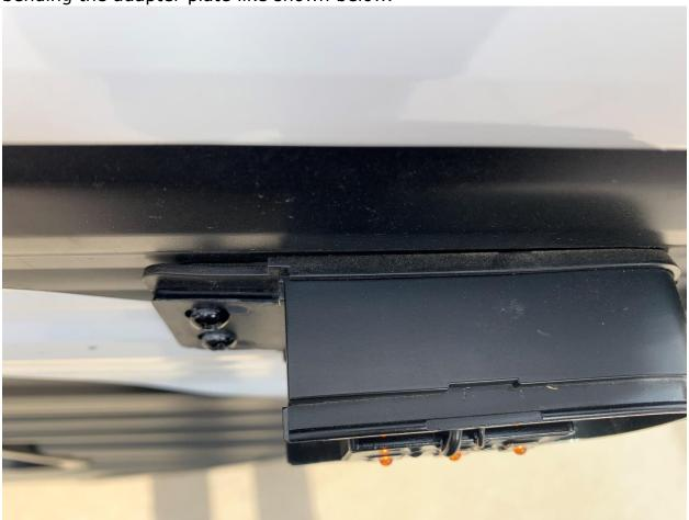
To correct, insert a small washer or other spacer between the plastic mount and the rubber gasket. Resecure these 2 screws. If it is flat already. Only loosen the 2 screws in the front of the marker.
