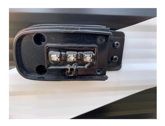
Losen the 4 Phillips screws. The 2 facing the rear of the RV are likely bending the adapter plate like shown below.
